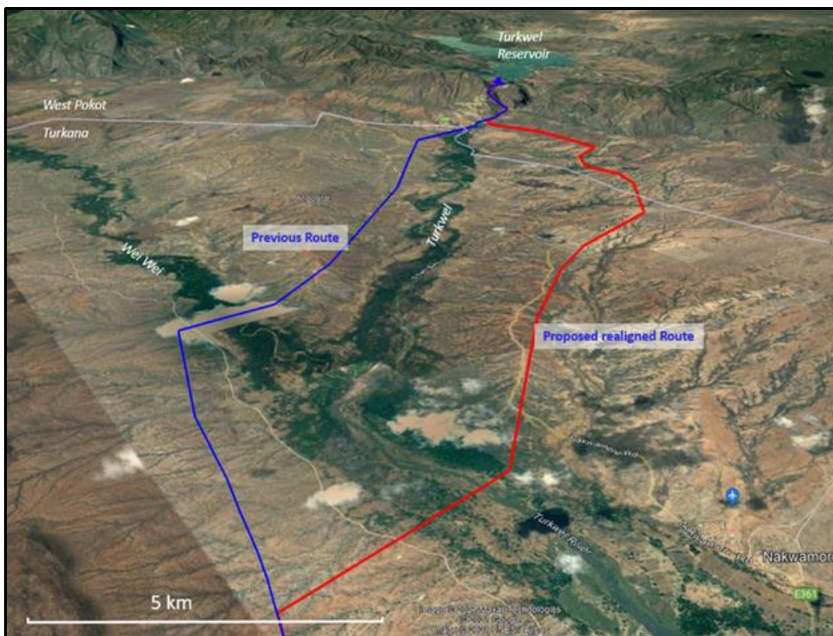
Figure 5.1 Original and Revised Water Supply Pipeline Routes
